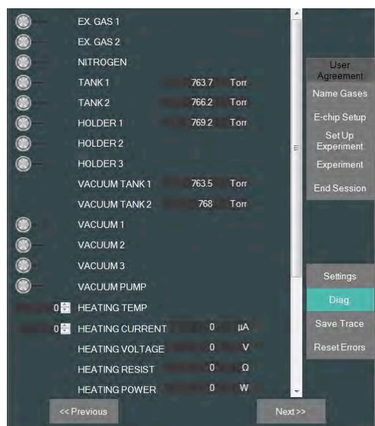
FIGURE 34. THE DIAGNOSTICS SCREEN. THE TEMPERATURE, VACUUM PUMP AND EACH VALVE CAN BE INDEPENDENTLY CONTROLLED HERE.
