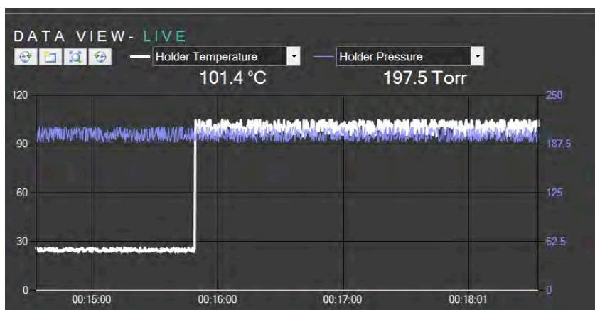
FIGURE 29. THE DATA VIEW SCREEN. DATA VIEW SHOWS A GRAPHICAL REPRESENTATION OF THE DATA AND LARGE TEXT SHOWING THE CURRENT STATUS OF THE SYSTEM PRESSURE AND/OR HOLDER TEMPERATURE.
