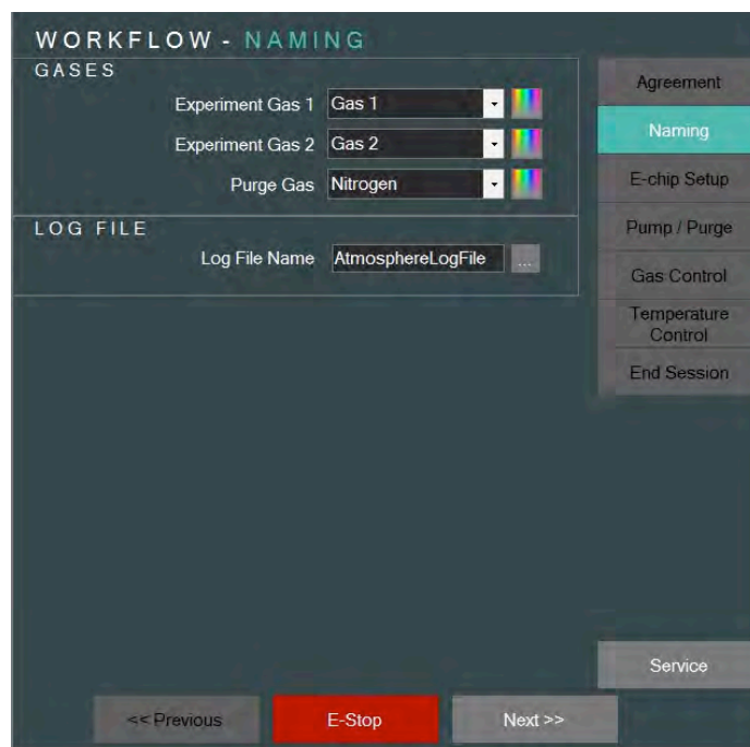
FIGURE 17. THE NAME GASES SCREEN, WHERE EACH INPUT GAS CAN BE NAMED AND COLOR CODED.
